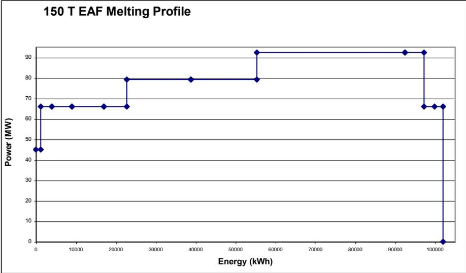
Figure 2. Melting Practice with respect to Power Input.
