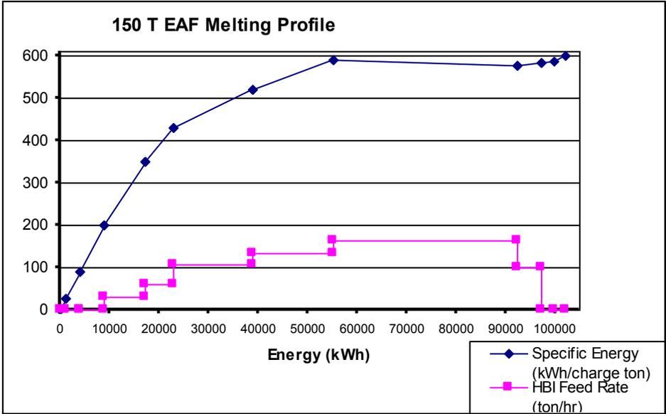
Figure 1. Melting Practice with Respect to Energy Input and HBI Feed Rate.
